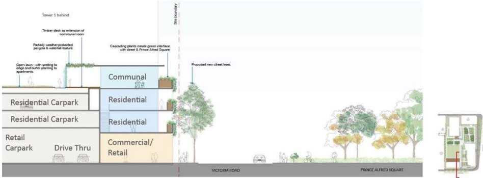
Figure 60 - Excerpt showing a detail of the Reference Design through the podium. (Source: Bates Smart)
